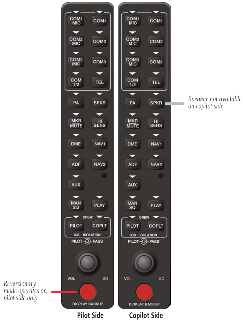
Figure 6A.3.9 Dual G1000 Audio Panels (GMA 1347)
