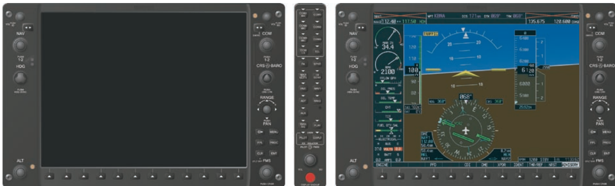
Figure 1-9 Reversionary Mode (Failed PFD)
